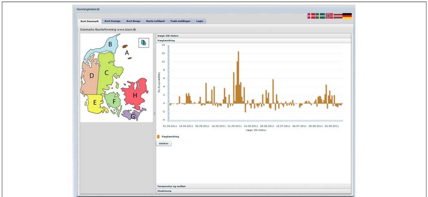
Fig. 19. The Nordic/baltic honey meter. Over 66 scales are distributed in four countries (Denmark, Sweden, Norway, Latvia). Here food/honey consumption/weight gain for the period 1.4.2011-1.9.2011 is shown for a scale located close to the town Hobro in Jutland, Denmark.
