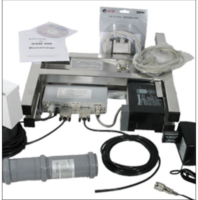
Fig. 15. The Capaz scale is an H-shaped platform made from aluminium and stainless steel, with the dimensions 420 x 480 x 86 mm (long x wide x high). Data are transmitted by cell phone. The rechargeable battery (12 V) lasts for 200 days. Ambient temperature and humidity are measured by default. Additional equipment is the rain collector and brood temperature sensor. Changes of the standard setup of the scale are done via the computer software. Photo: Capaz.
