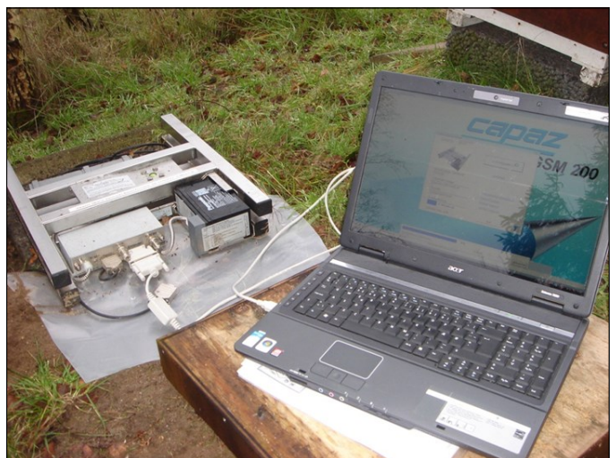
Fig. 16. Configuration of the Capaz scale directly in the apiary.
